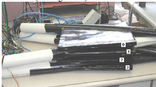
Figure 30. Shown here is a four-counter setup used in plateauing counters using the multiple counter method. Each counter is paired with another and coincidences are plotted over increasing voltages.
