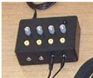
Figure 14. Power distribution unit. One black and four yellow test points allow one to check voltage on the PMTs.
