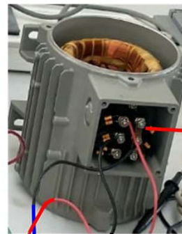
Stator of two-phase electric power
